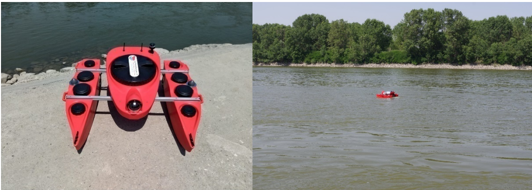
Figure 7: Proambiente's Unmanned Survey Vehicle, during the field measurement session at Po River during W.A.T.E.R. 2019.
