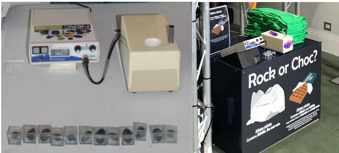
235 Figure 3: Rock or Choc setup, with boxes of chocolate and rock pebbles, and a Bartington susceptibility meter.
