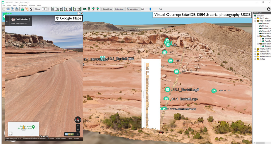
925 Figure 5. Bartlett Wash, Utah, USA, model available on SafariDB . The task at this locality is to interpret the depositional environment and consider reservoir compartmentalisation. Virtual outcrop from SafariDB and viewed in LIME with additional material including logs, photos, and 360 photo spheres (in this example from ©Google Maps). Aerial Photography on DEM, USGS EROS Archive; DEM, USGS 3D Elevation Program.
