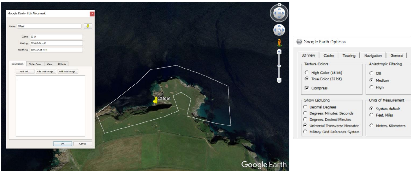
Figure 6. Use a GIS or earth viewer such as Google Earth to define coordinate offsets for model processing and export.
