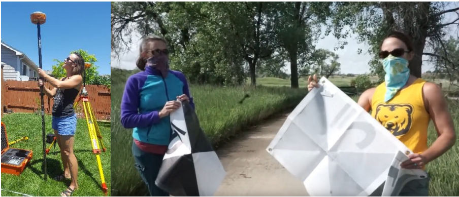
657 658 Figure 2. Base and Kinematic GNSS methods (left) and example of ground control (right) surveyed for use in GNSS and SfM 659 activities.
