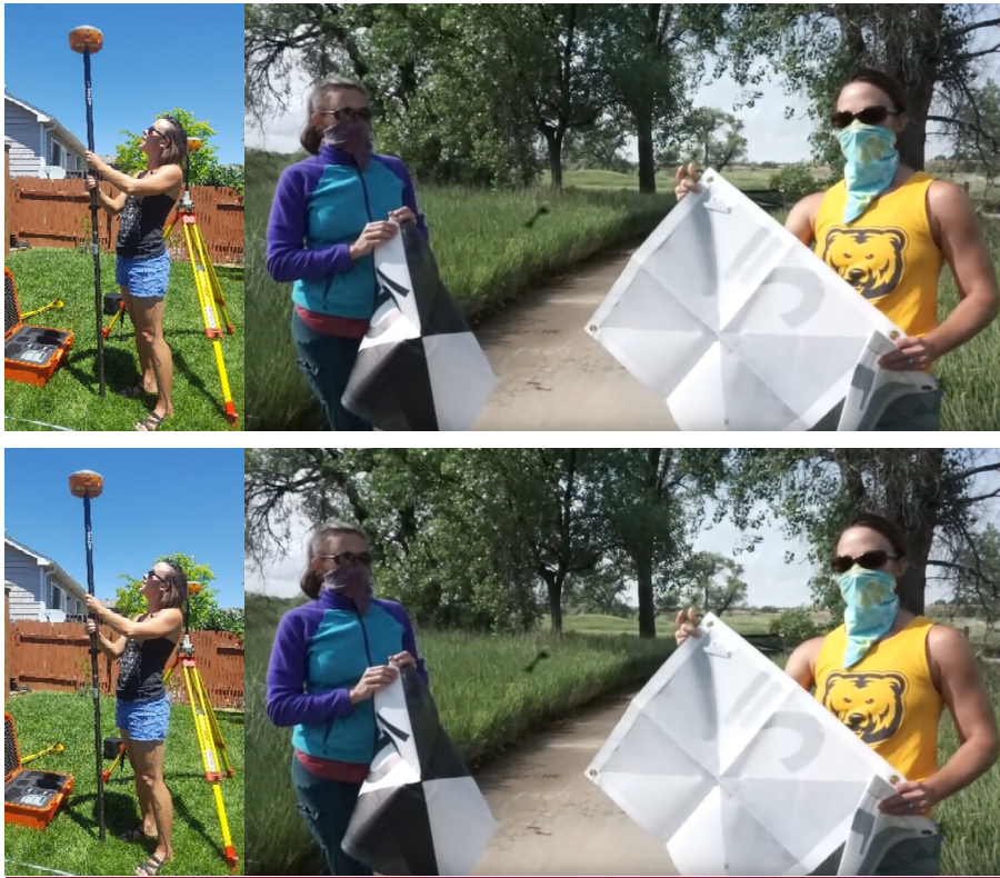
Figure 42. Base and Kinematic GNSS methods (left) and example of ground control (right) surveyed for use in GNSS and SfM activities.
