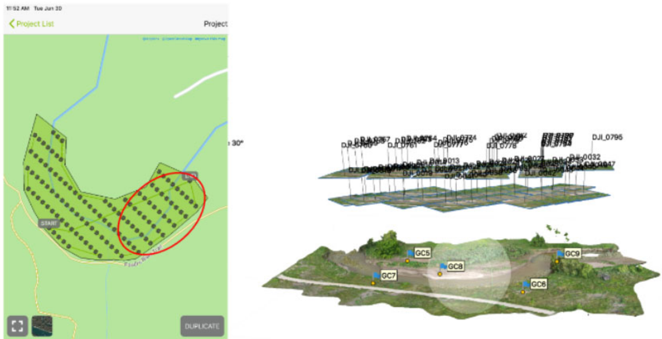
Figure 5. Example of a student's area of interest (left) picked and associated MetaShape georeferenced point cloud (right) of their area of interest (created by student in course; student not disclosed to comply with Institutional Review Board).
