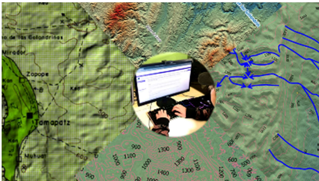
300 Figure 7. Advanced activity synthesis, clockwise from left: analog geological map draped over topography using QGIS, DEM with hillshade in QGIS, manually drawn flow routing, and elevation contour layers in QGIS. Photo by author.
