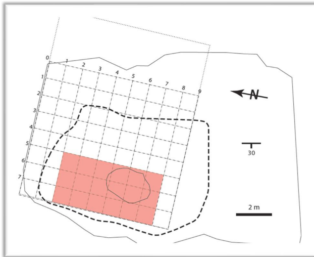
Figure 3. Grid layout used to take photographs. The grid spacing is 1 m, and photos were taken from each grid intersection with a camera aimed into the target grid space. The shaded area shows the area we processed for this study, and the heavy dashed line outlines the map area from Kappus et al. (2011).
