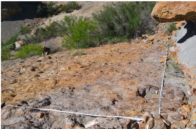
Figure 4. The grid system used in this study was based on two metric tape measures laid out perpendicular to each other to establish the locations for photographs. The positions of the individual grid intersections at 1 m spacing were marked as shown in Fig. 5.
