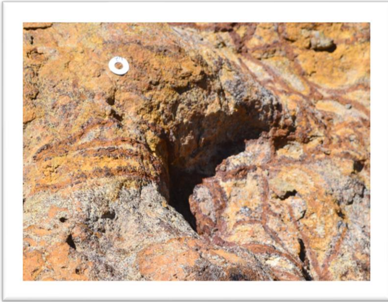
350 Figure 5: Shows the circular mark used to indicate the intersection of two 1-m spaced grid lines in the survey area.
