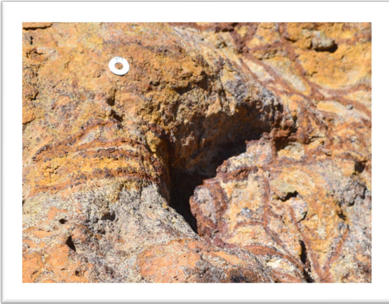
410 Figure 5 Showing the mark that indicates the intersection of two 1-m spaced grid lines in the survey area.
