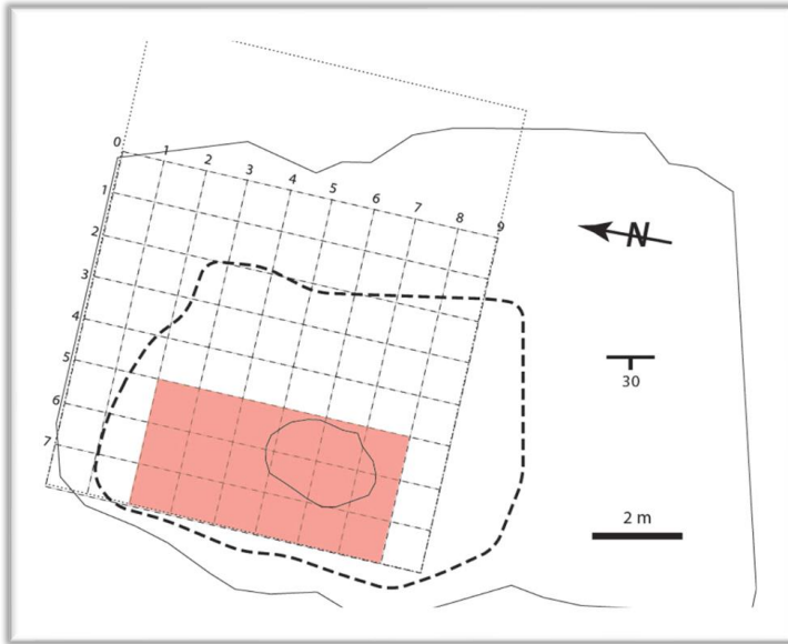
Figure 3 Grid layout used to take photographs. The grid spacing is 1 meter and photos were taken from each grid intersection with a camera aimed into the target grid space. The shaded area shows the area we processed for this study and the heavy dashed line outlines the map area from Kappus et al.(2011).
