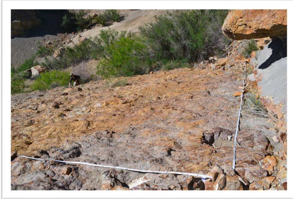
Figure 4 The grid system used in this study was based on 2 metric tape measures laid out perpendicular to each other to establish the locations for photographs. The position of the individual grid intersections at 1 meter spacing was marked as shown in Figure 5.
