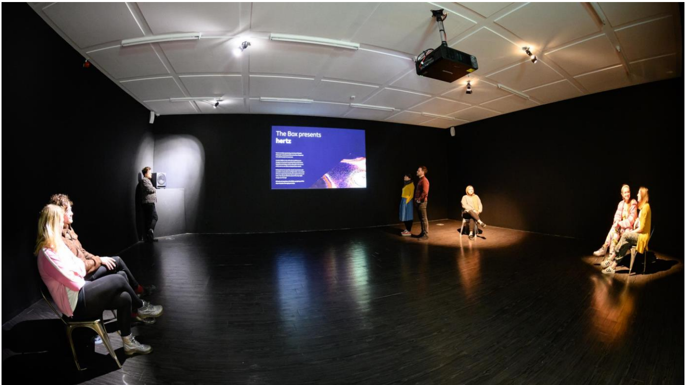
685 Figure 10: Finalised version of the hertz infrasound installation at the box at We the Curious Bristol. Members of the public sit on the furniture which has transducers beneath. The subwoofer is located in the far-left hand corner. Information about hertz is projected on to the wall
