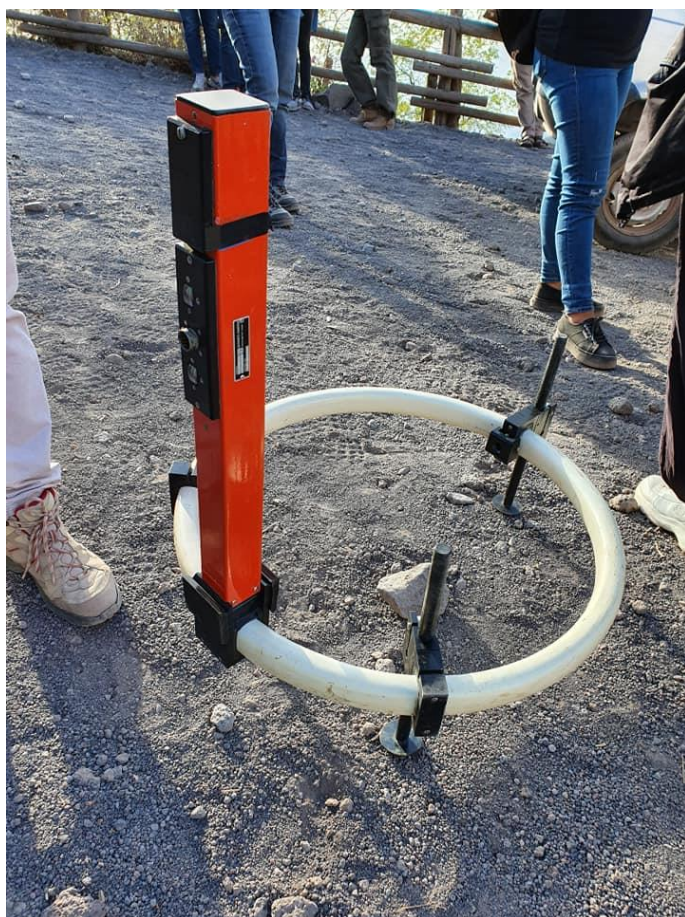
Figure 2: The receiver coil that records the Earth EM response.
