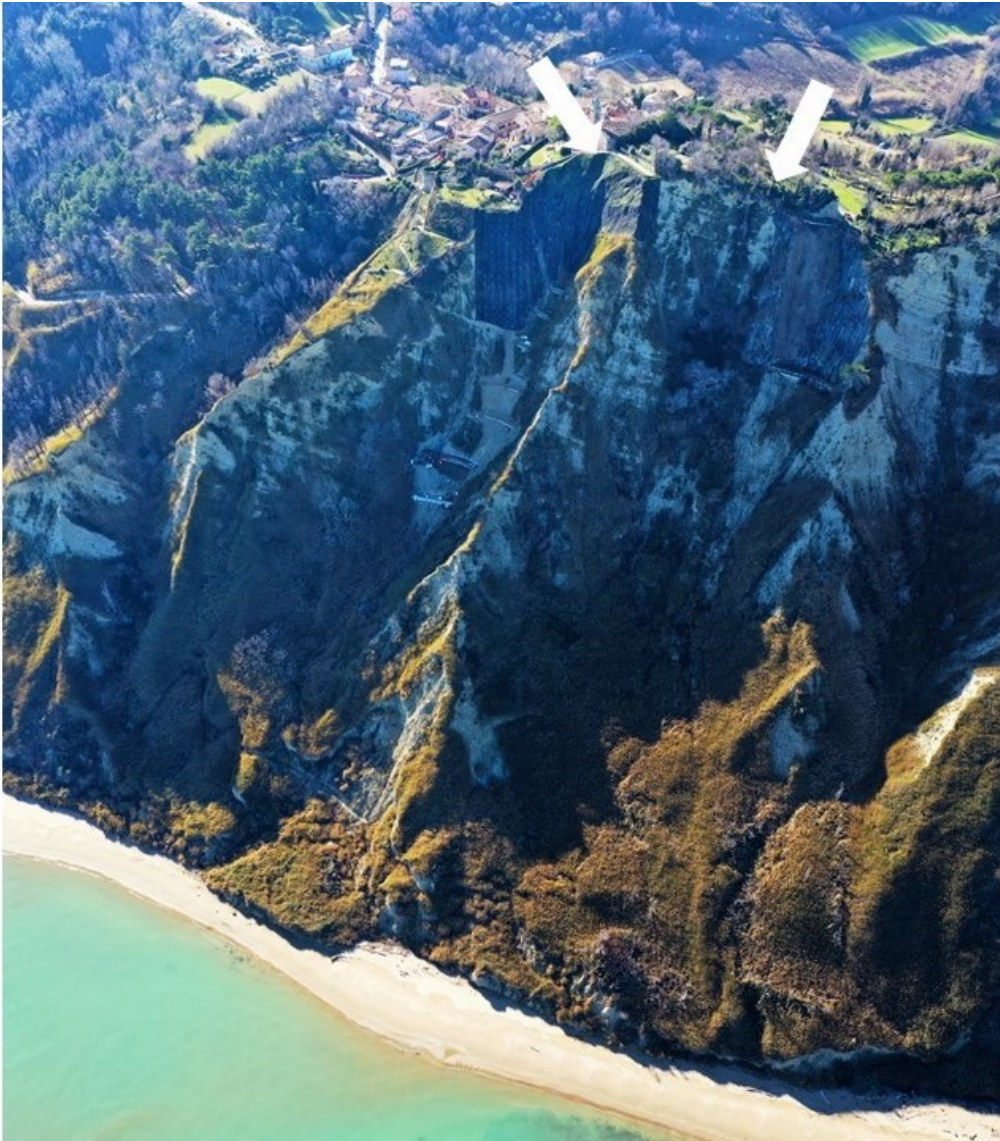
Figure 4: Panoramic view of the active cliffs of Mount San Bartolo. The cliff is oriented NW (on the right) – SE (on the left); the small village of Fiorenzuola di Focara (on the top of the cliff) is 177 m asl. The arrows indicate the landslide scarps.
