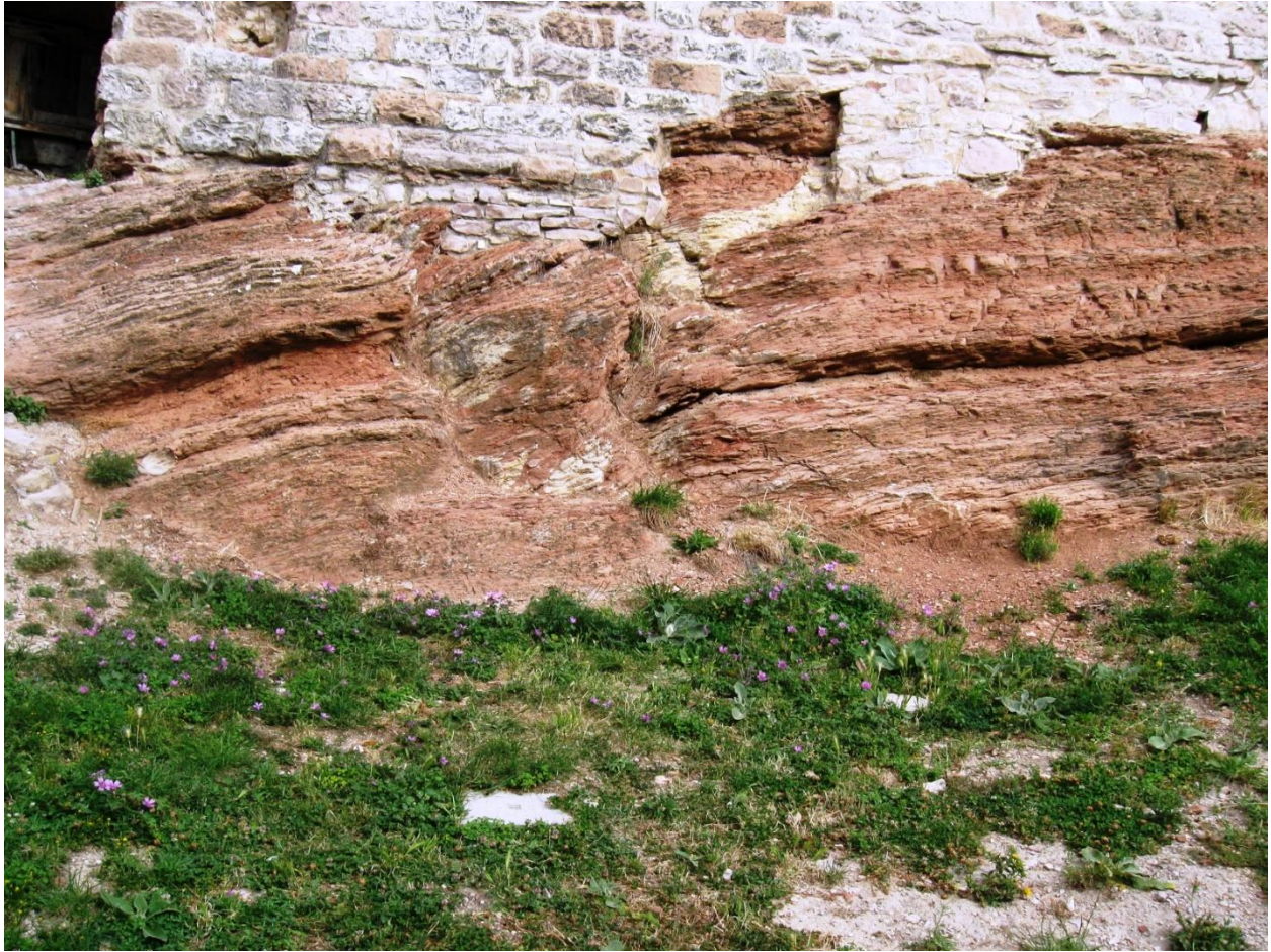
Fig. 2. Pink streaked with white Scaglia Rossa limestone is a pelagic sedimentary rock with forams and clay in a coccolith matrix dating from the Late Cretaceous to middle Eocene. Mined from the Mt. Subasio quarry and used to construct the St. Francis basilica at Assisi. Public domain Wiki Commons
