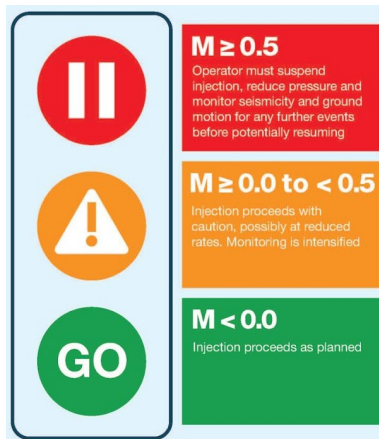
587 588 Figure 1: The UK's traffic light system for regulating induced seismicity from hydraulic fracturing activities for shale 589 gas extraction, figure from DECC (2013b), made by the Oil and Gas Authority. The traffic light system is based on a 590 risk mitigation technique originally developed for geothermal (Cremonese et al., 2015). It requires operators to
