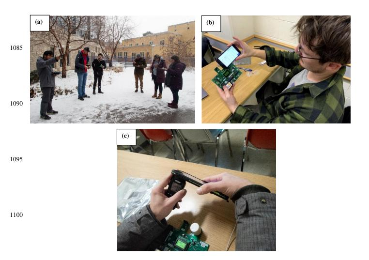
1105 **Fig. 9.** Students engaged in calibration activities. (a) Outdoor calibration of temperature, RH and pyranometer devices using hand-held commercial sensors. Indoor calibration (b, c) with a smartphone flashlight and a hand-held solar radiation meter used as a standard for comparison.
