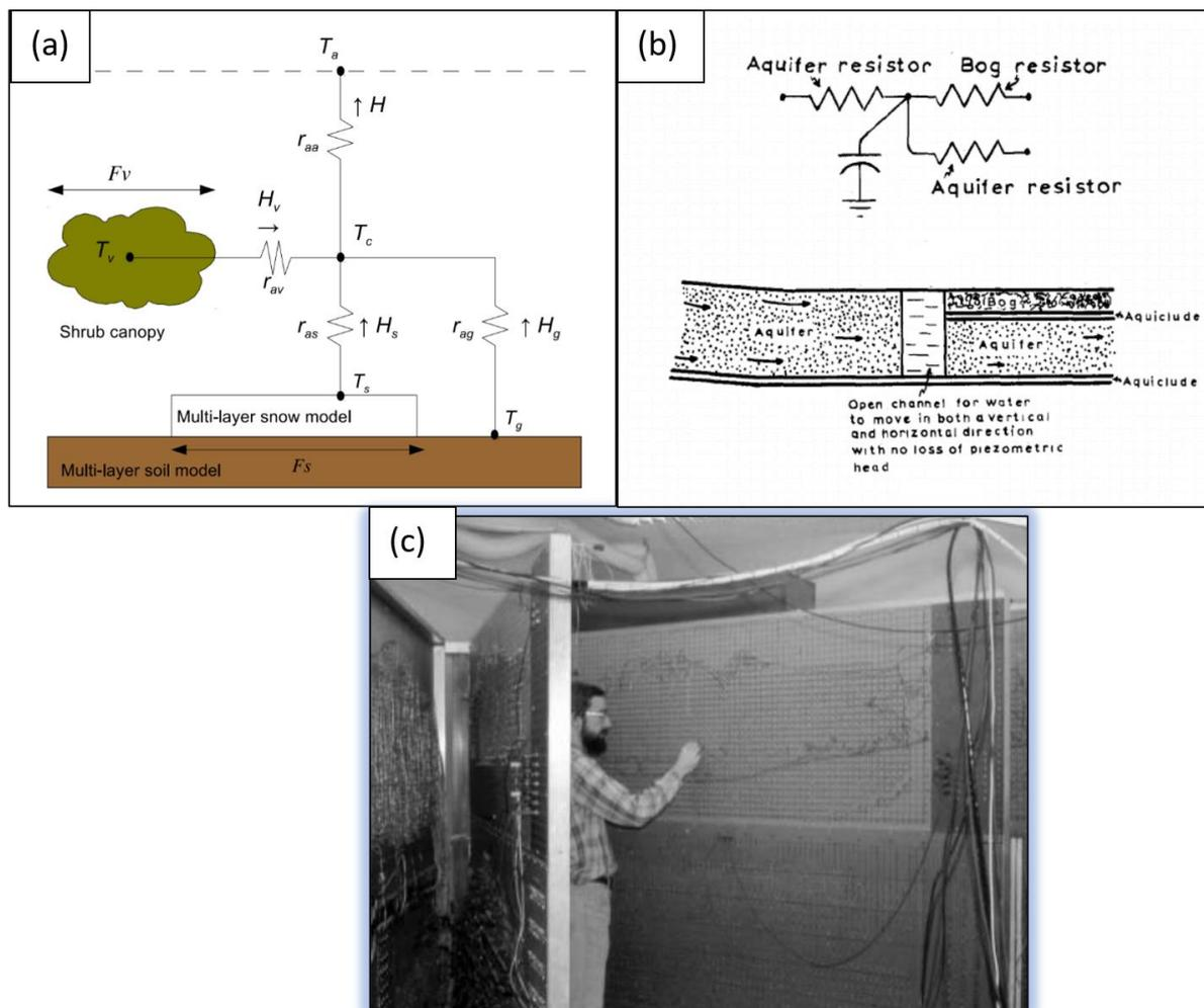
885 **Fig. 2.** (a) Example of an analog model used for modelling heat exchange between snow, soil, a shrub canopy and the
