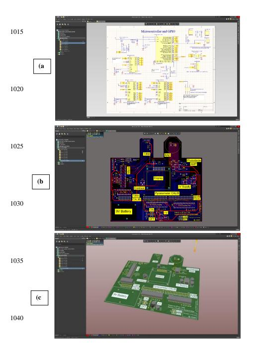
Fig. 7. (a) Layout software showing a schematic page of the hybrid temperature, relative humidity, and solar radiation sensor. (b) Associated circuit board with layers stacked in a similar fashion to a geographic information system (GIS). (c)
