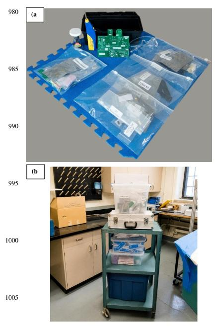
Fig. 6. (a) The circuit components were individually bagged and labelled for student assembly. Also visible in this image is the battery-operated soldering iron used by students for soldering, a toolbox containing hand tools for assembly and a glue
