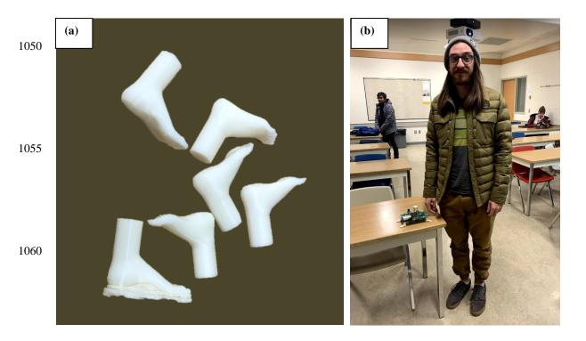
1065 Fig. 8. (a) Example of 3D printed "feet" to be glued on the bottom of a PCB. The 3D printed "foot" nearest the bottom of the image has a 3D printed "raft" that has not been removed. The "raft" is placed on the 3D printer build platform to ensure that the deposited plastic sticks to a substrate. (b) Student next to a PCB exhibiting "feet" glued on the bottom.
