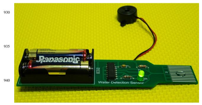
**Fig. 4**. Water detection PCB. A droplet of water turns on the light-emitting diode (LED) and an attached piezoelectric buzzer to provide visual and audible feedback.
