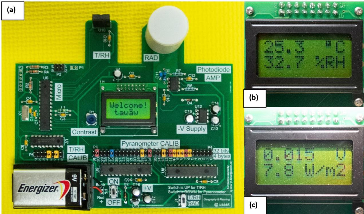
**Fig. 5.** (a) Hybrid temperature, relative humidity (RH) and solar radiation sensor. (b) LCD display showing calibrated
