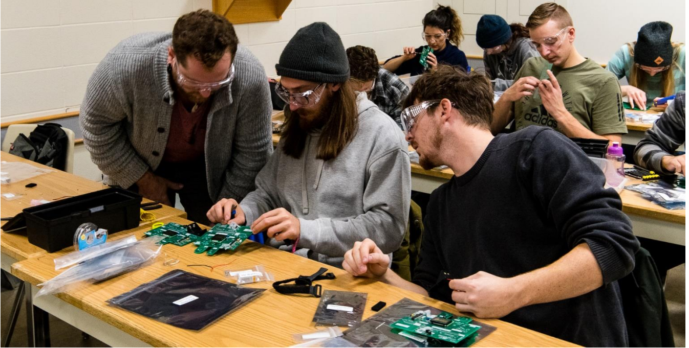
Fig. 6. Example images of circuit assembly in the class. The students are using battery-operated soldering irons to solder components to the PCB.
