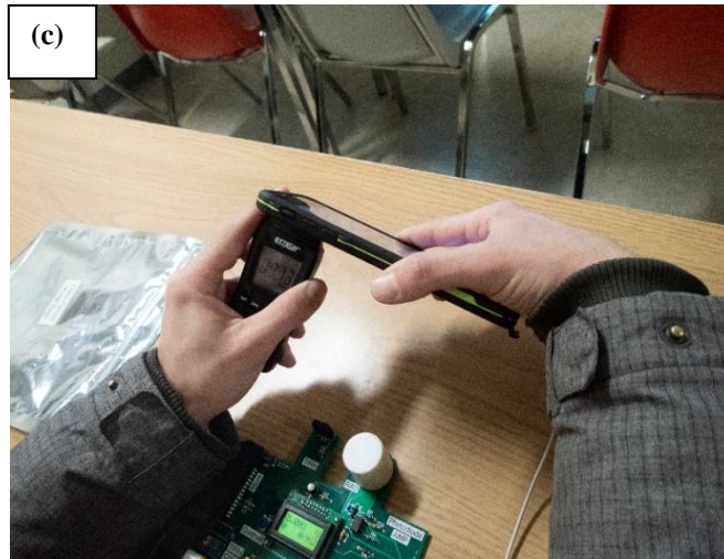
1115 Fig. 9. Students engaged in calibration activities. (a) Outdoor calibration of temperature, RH and pyranometer devices using hand-held commercial sensors. Indoor calibration (b, c) with a smartphone flashlight and a hand-held solar radiation meter used as a standard for comparison.
