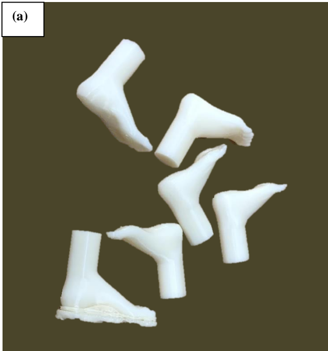
Fig. 10. (a) Example of 3D printed “feet” to be glued on the bottom of a PCB. The 3D printed “foot” nearest the bottom of the image has a 3D printed “raft” that has not been removed. The “raft” is placed on the 3D printer build platform to ensure that the deposited plastic sticks to a substrate. (b) Student next to a PCB exhibiting “feet” glued on the bottom.
