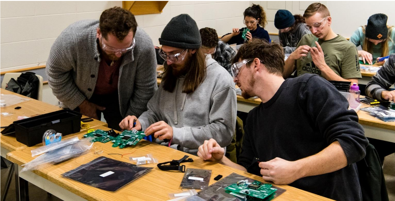
Fig. 6. Example images of circuit assembly in the class. The students are using battery-operated soldering irons to solder components to the PCB.
