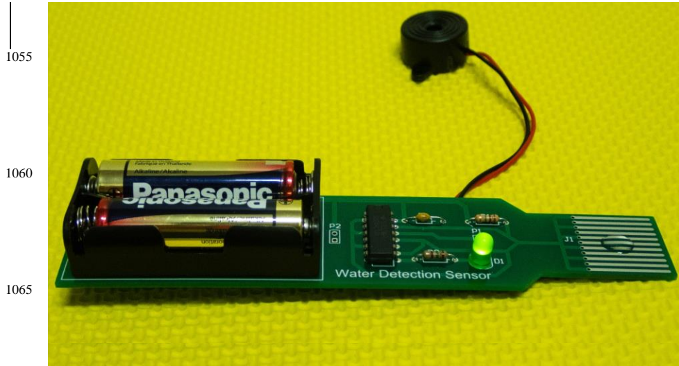
1070 Fig. 7. Water detection PCB. A droplet of water turns on the light-emitting diode (LED) and an attached piezoelectric buzzer to provide visual and audible feedback.
