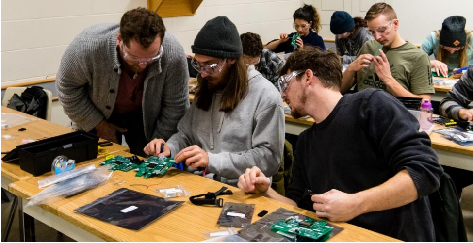
1035 Fig. 6. Example images of circuit assembly in the class. The students are using battery-operated soldering irons to solder components to the PCB.
