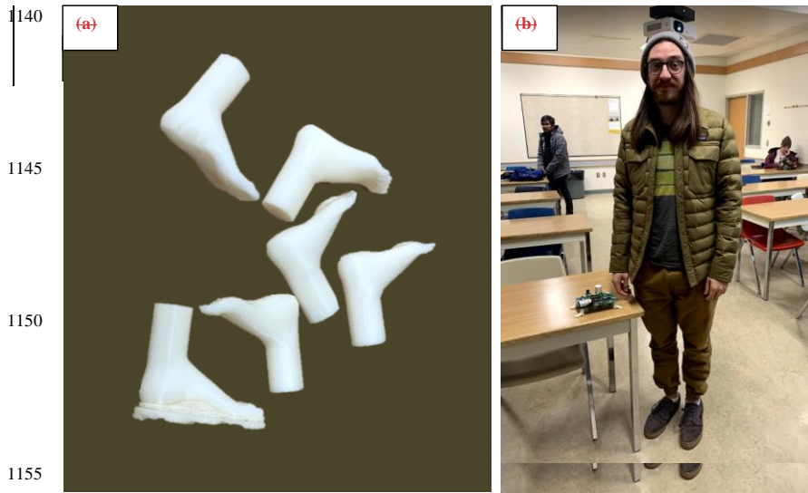
Fig. 10. (a) Example of 3D printed “feet” to be glued on the bottom of a PCB. The 3D printed “foot” nearest the bottom of the image has a 3D printed “raft” that has not been removed. The “raft” is placed on the 3D printer build platform to ensure that the deposited plastic sticks to a substrate. (b) Student next to a PCB exhibiting “feet” glued on the bottom.
