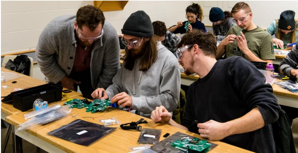
Fig. 36. Example images of circuit assembly in the Advanced Hydrology class. The students are using battery-operated soldering irons to solder components to the PCB.
