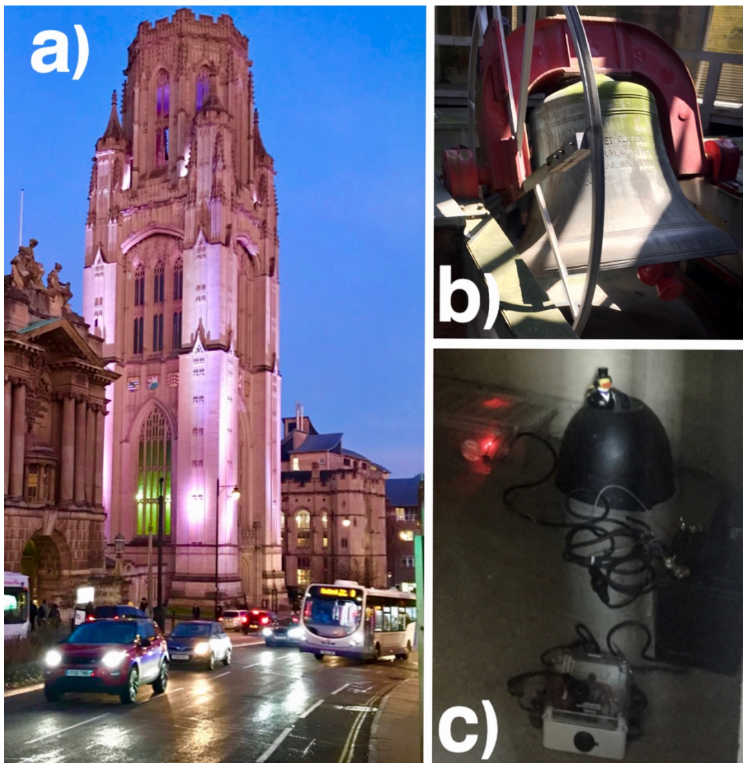
660 Figure 1: Great George Bell (b) sits within the belfry of the Wills Memorial Building pictured in (a) on a typical weeknight. The broadband seismometer (c) installation setup in one of the alcoves above the bell. The instrument itself lies beneath the black dome with the Brunel rubber duck (geophysics group mascot) on top.
