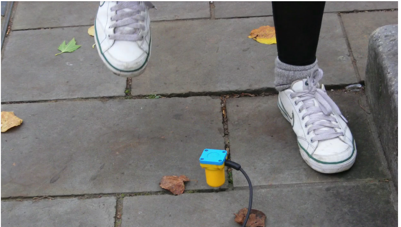
750 Figure 2: Workshop participant jumping near geophone set up to record foot traffic near the Wills Memorial Building
