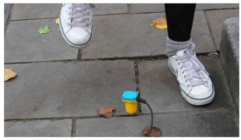
Figure 2: Workshop participant jumping near geophone set up to record foot traffic near the Wills Memorial Building
