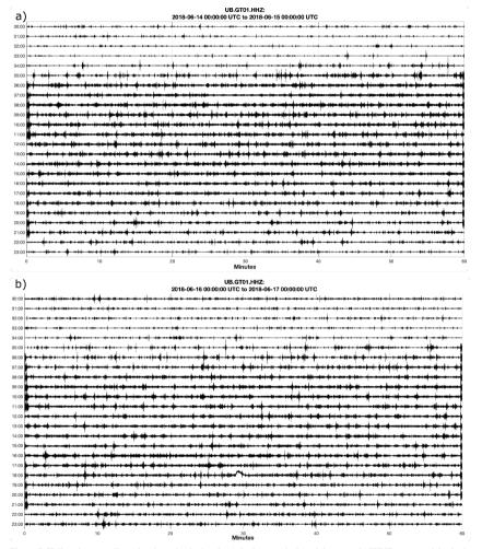
1025 Figure 5: Helicorder recordings showing seismic signals (a) during a typical weekday near the WMB tower and (b) during a Saturday evening near the tower. During the week, while never fully quiet, activity tends to wane at night around 10 PM in contrast to a weekend night when activity is heightened until about 3 AM.
