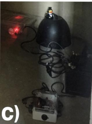
1000 Figure 1: Great George Bell (b) sits within the belfry of the Wills Memorial Building pictured in (a) on a typical weeknight. The broadband seismometer (c) installation setup in one of the alcoves above the bell. The instrument itself lies beneath the black dome with the Brunel rubber duck (geophysics group mascot) on top.
