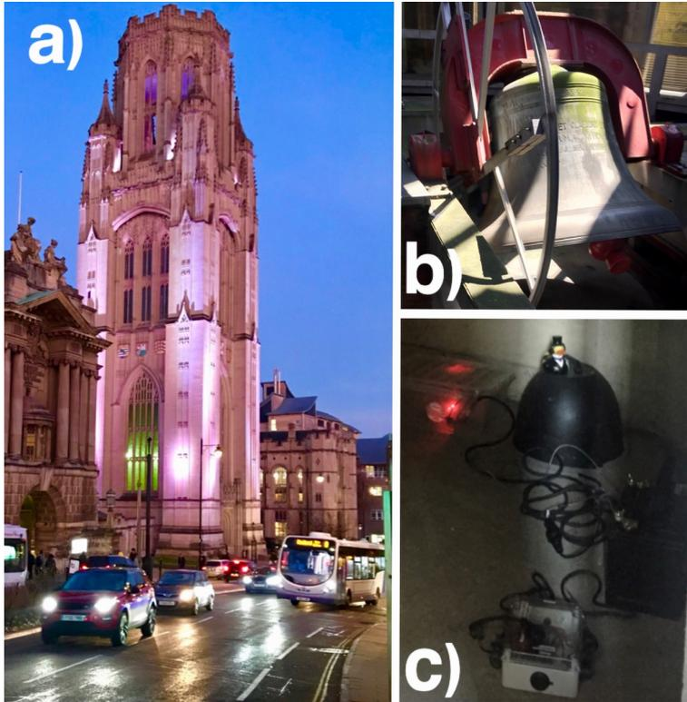
1000 **Figure 1:** Great George Bell (b) sits within the belfry of the Wills Memorial Building pictured in (a) on a typical weeknight. The broadband seismometer (c) installation setup in one of the alcoves above the bell. The instrument itself lies beneath the black dome with the Brunel rubber duck (geophysics group mascot) on top.
