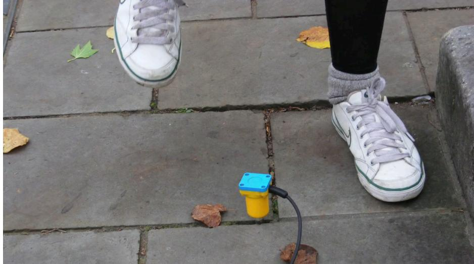
Figure 2: Workshop participant jumping near geophone set up to record foot traffic near the Wills Memorial Building
