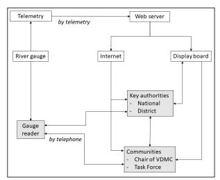
Figure 2. Risk information communication including telemetry system and actors (in grey) (from Gurung, 2016)
