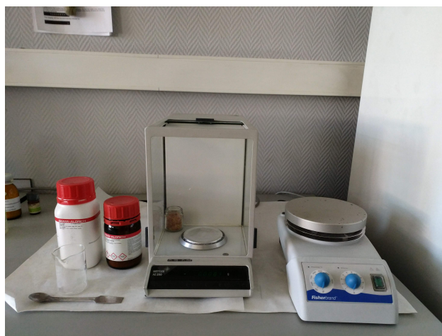
Figure 3. Instrumentation and materials (potassium iodide (KI), starch ( C_6H_{10}O_5 ), rods, beakers, balance and stove)
