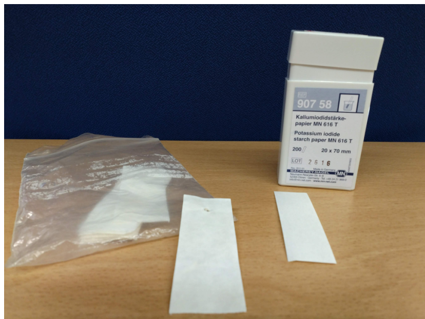
Figure 6. Example of strips (left: made by ourselves, right: comercial strips).
