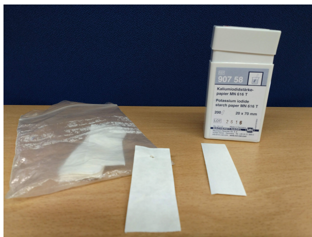
Figure 4. Example of strips (left: made by ourselves, right: commercial strips)
