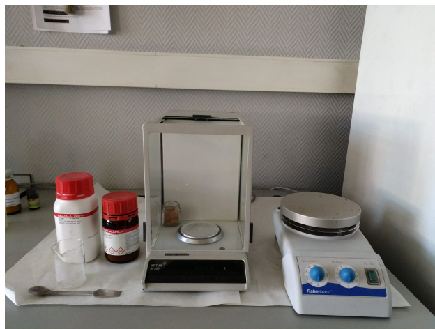
Figure 3. Instrumentation and materials (potassium iodide (KI), starch (( C_6H_{10}O_5 ), rods, beakers, balance and stove)
