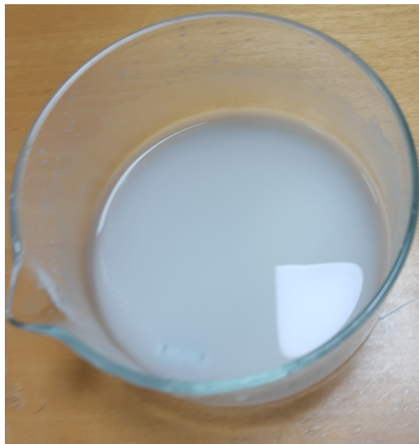
Figure 5. Mixture resulting from the solution of KI and starch in hot distilled water.
