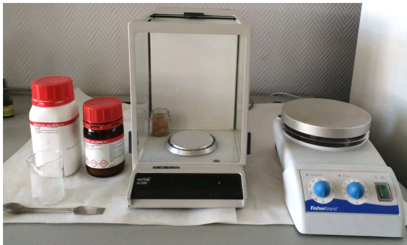
Figure 4. Instrumentation and materials (potassium iodide, starch, rods, beakers, balance and stove).
