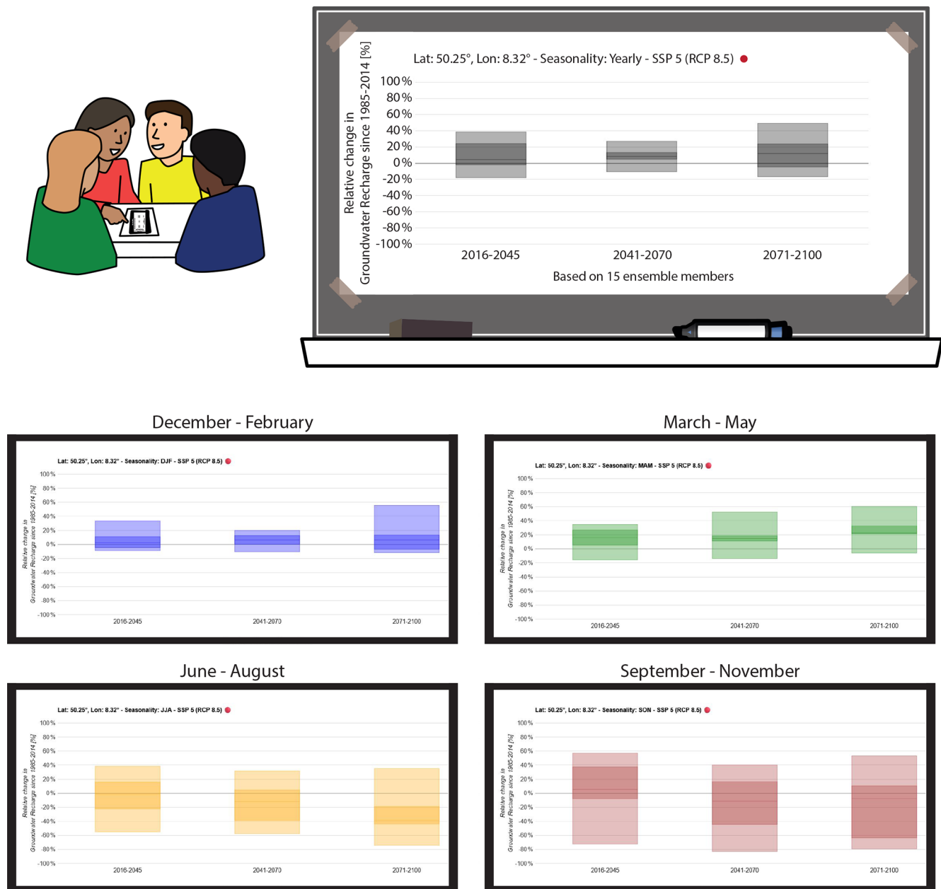
Figure 3. Arrangement of five downloaded png files with “Local Insights” plots for the 0.5° grid cell north of Frankfurt (Germany), where the municipality of Waldems is located. It may serve to inform local stakeholders about potential future changes in groundwater recharge. The arrangement shows, at the top, the changes in annual groundwater recharge between the reference period and three future time periods, and, below, the projected changes in seasonal groundwater recharge.
