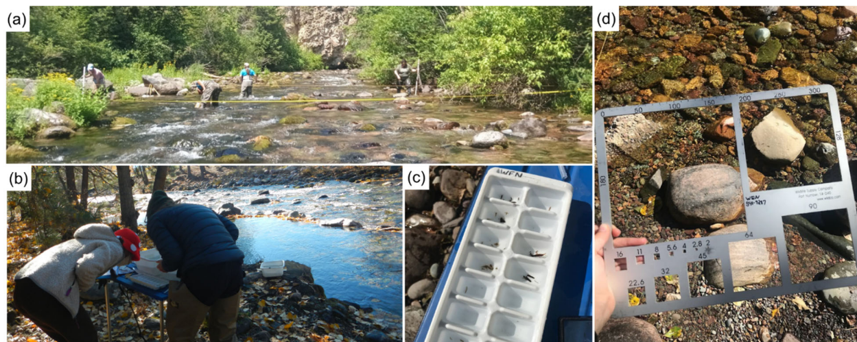
Figure S1. Photos of the Watershed Education Network Stream Team monitoring. Methods include measuring cross-sectional profiles (a), conducting aquatic macroinvertebrate counts (b, c), and conducting pebble counts (d). Photos courtesy of Stephie Novak (WEN; a-c) and Bethany Blakey (d).
