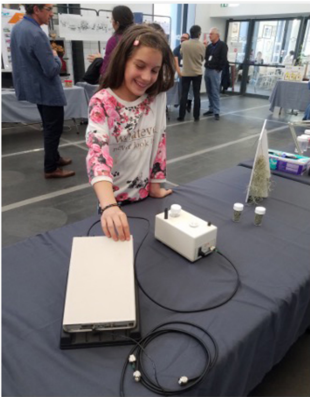
Figure 4. Child performing measurements of bark samples in Component 3 with a susceptibility meter. Photo credit: Melina Macouin. Image reproduced with permission from the child’s legal guardians.
